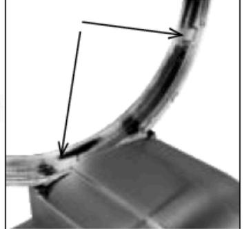
Two nylon pads were used on clocks made after 1955 to reduce friction from the glass and gear ring riding on the dial frame.
